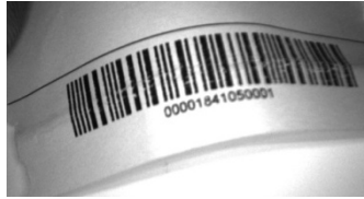
Figure 20 - Barcode Printed on Curved Surface Readable despite Optical Distortion
