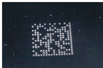
Figure 23 - Directly Marked Dot Matrix Code Characterized by Outstanding Separation Distance between Adjacent Code Elements
