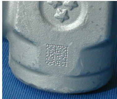
Figure 21 - Dot Matrix Code Directly Marked on Metal Surface by Using Dot Peening Technology
