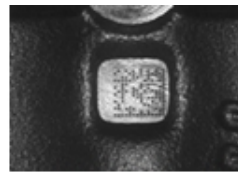
Dot Peening On Scratched Surface
